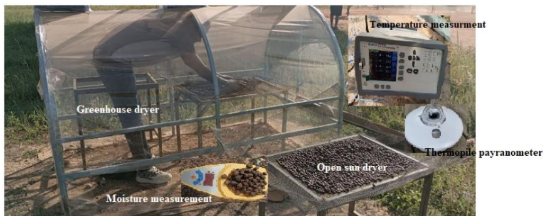
Figure 2. The manufactured integrated solar Coffee dryer.
